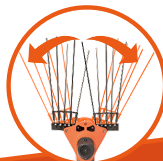
Working range 600 mm 2 x 5 flexible carbon fibre rods of 330 mm Seagull wing shaped – two combs with opposed movement
